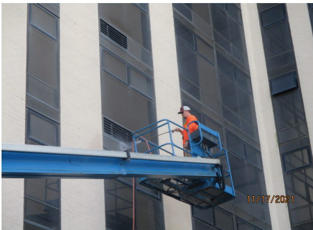
63. SPECIMEN 2.03: VIEW OF PCI PERSONNEL PERFORMING WATER SPRAY TESTING AT PERIMETER OF WINDOW
