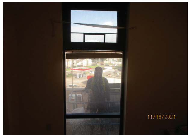
70. SPECIMEN 3.02: VIEW OF PCI PERSONNEL PERFORMING WATER SPRAY TESTING AT PERIMETER OF WINDOW
