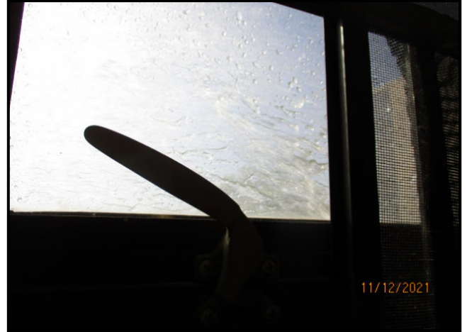
50. SPECIMEN 1.01: VIEW OF PCI PERSONNEL PERFORMING WATER SPRAY TESTING AT PERIMETER OF WINDOW
