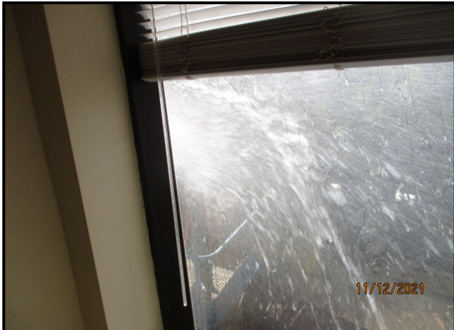
51. SPECIMEN 1.01: VIEW OF PCI PERSONNEL PERFORMING WATER SPRAY TESTING AT PERIMETER OF WINDOW
