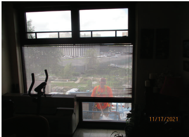
55. SPECIMEN 2.01: VIEW OF PCI PERSONNEL PERFORMING WATER SPRAY TESTING AT PERIMETER OF WINDOW
