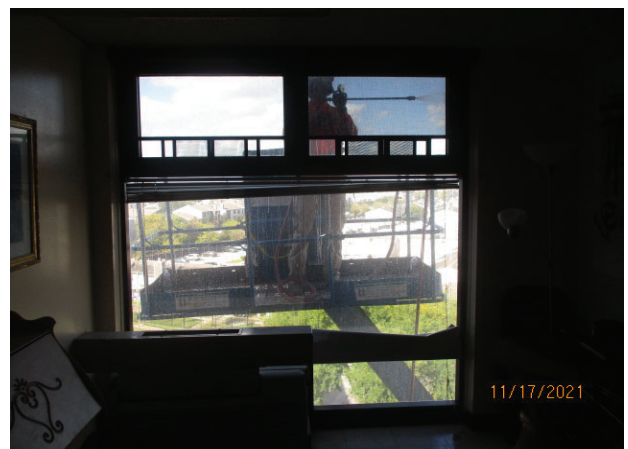
58. SPECIMEN 2.02: VIEW OF PCI PERSONNEL PERFORMING WATER SPRAY TESTING AT PERIMETER OF WINDOW
