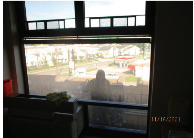
68. SPECIMEN 3.01: VIEW OF PCI PERSONNEL PERFORMING WATER SPRAY TESTING AT PERIMETER OF WINDOW
