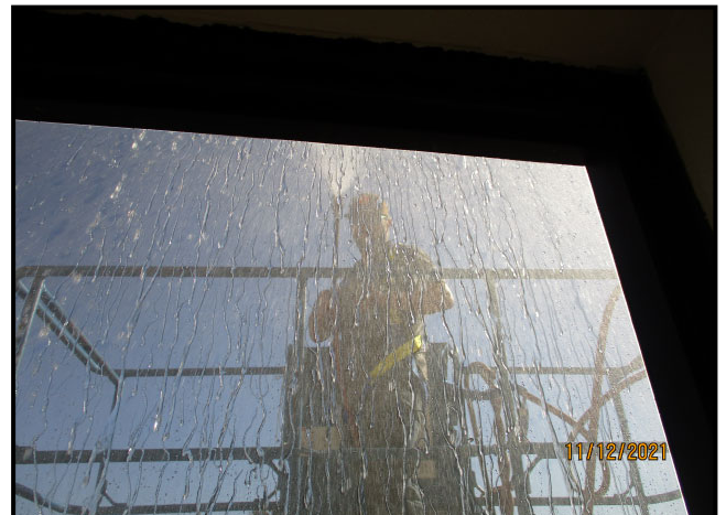
54. SPECIMEN 1.02: VIEW OF PCI PERSONNEL PERFORMING WATER SPRAY TESTING AT PERIMETER OF WINDOW
