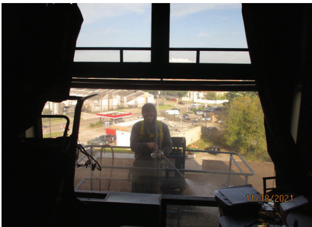
71. SPECIMEN 3.03: VIEW OF PCI PERSONNEL PERFORMING WATER SPRAY TESTING AT PERIMETER OF WINDOW
