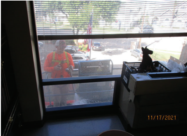
67. SPECIMEN 2.05: VIEW OF PCI PERSONNEL PERFORMING WATER SPRAY TESTING AT PERIMETER OF WINDOW
