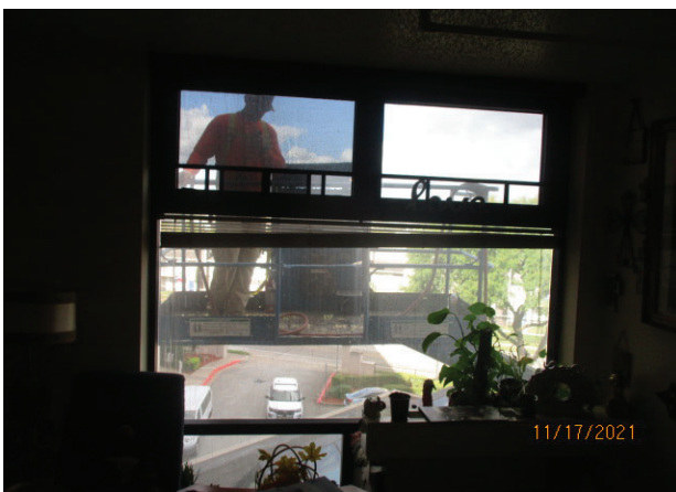
65. SPECIMEN 2.04: VIEW OF PCI PERSONNEL PERFORMING WATER SPRAY TESTING AT PERIMETER OF WINDOW
