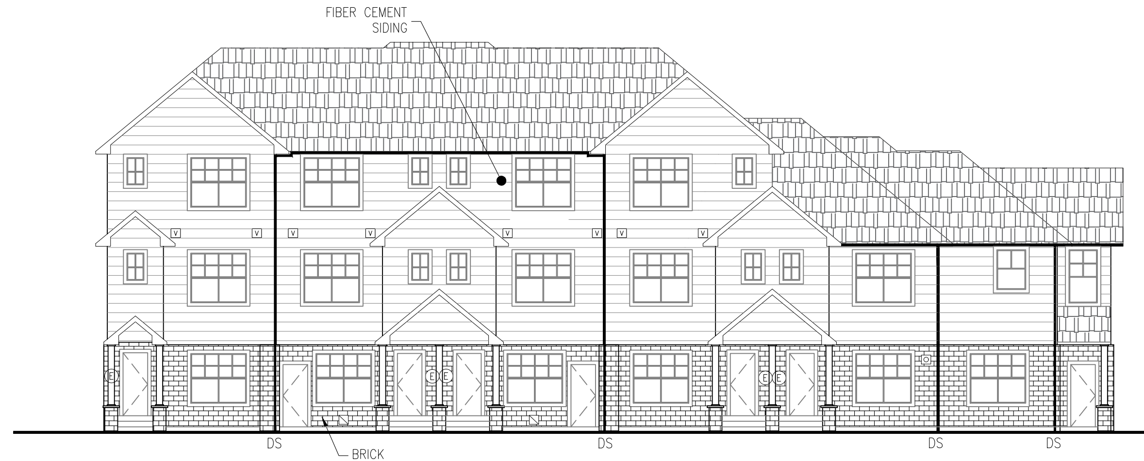
1 BUILDING 10 FRONT ELEVATION R3.07 NTS
