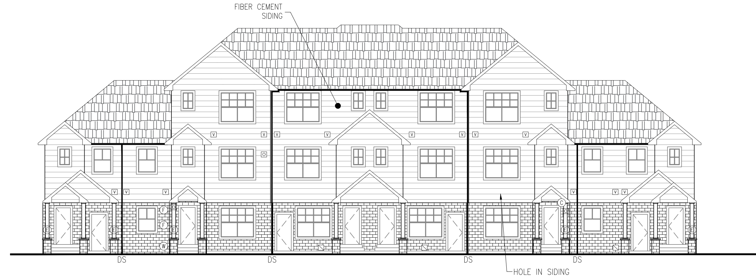
1 BUILDING 21 FRONT ELEVATION R3.18 NTS
