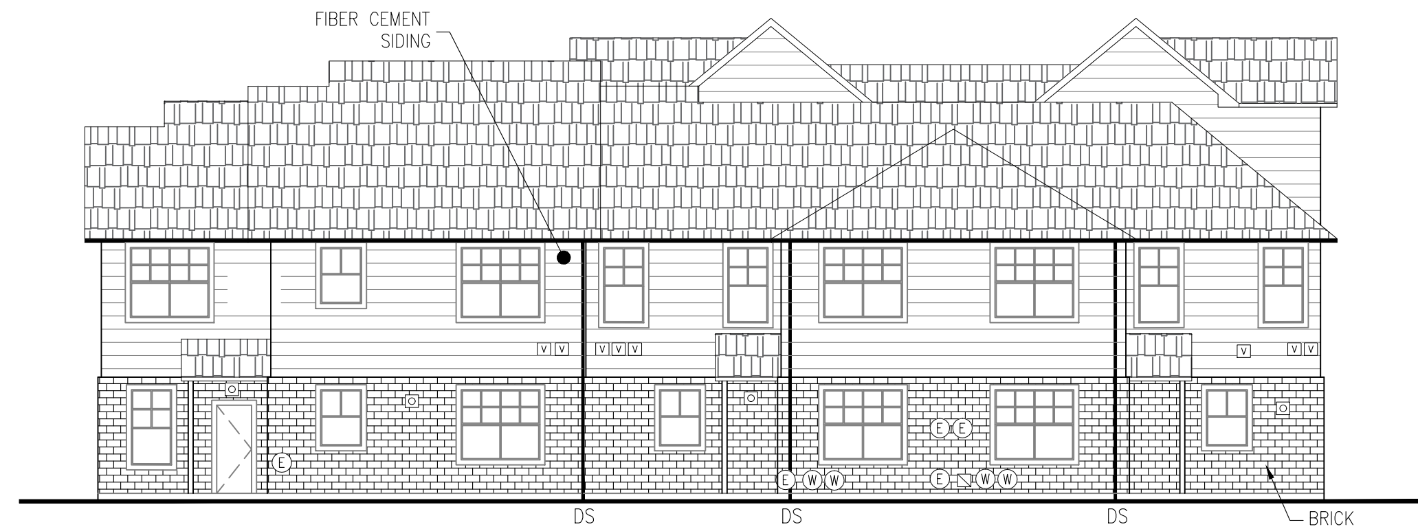
2 BUILDING 13 REAR ELEVATION R3.10 NTS
