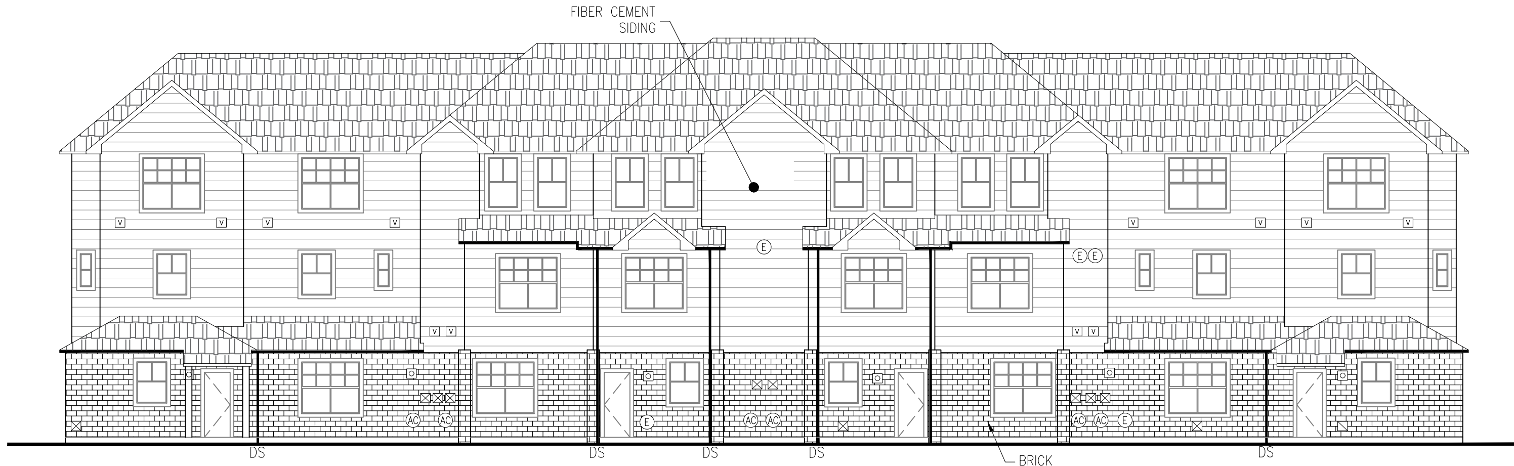
2 BUILDING 4 REAR ELEVATION R3.01 NTS
