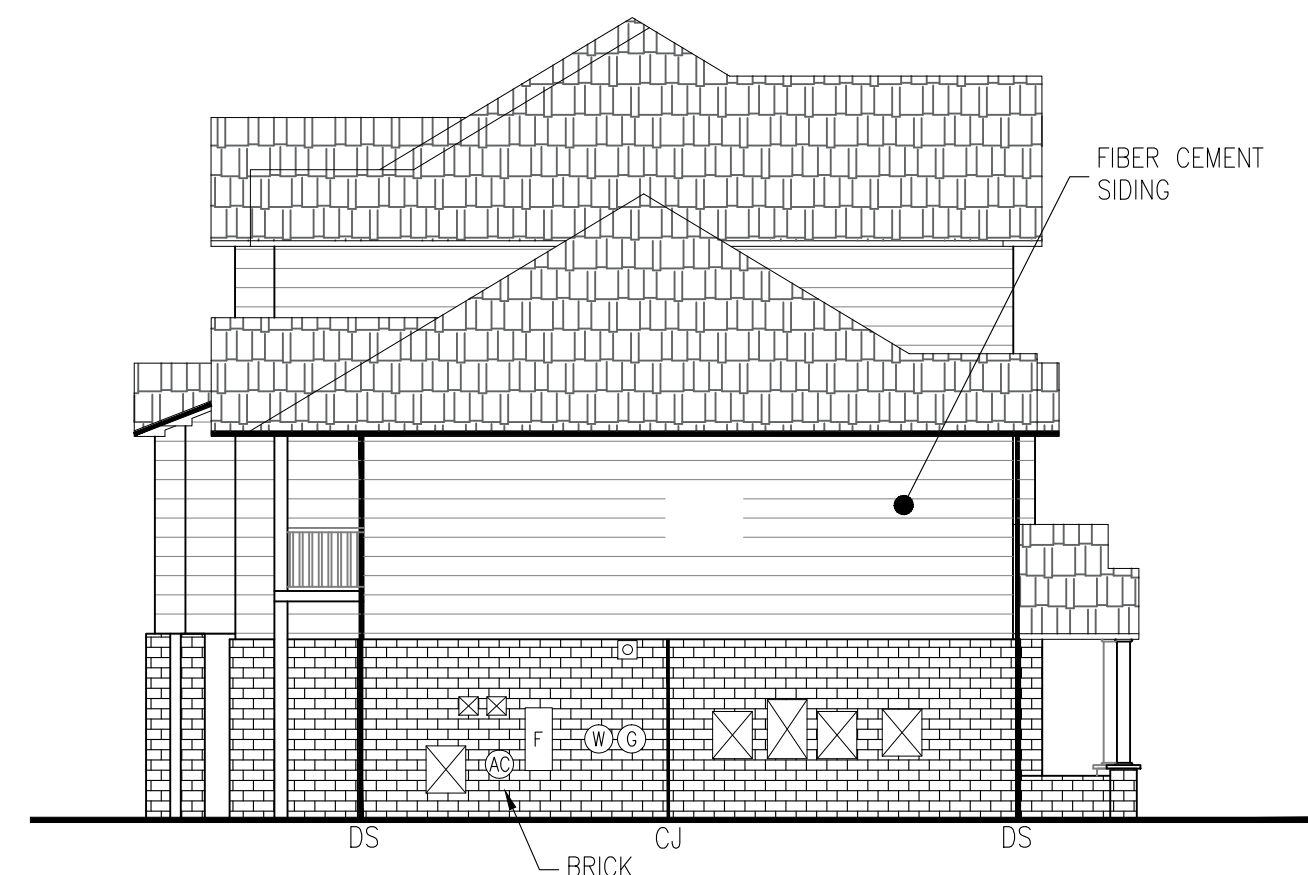
3 BUILDING 8 SIDE ELEVATION R3.05 NTS
