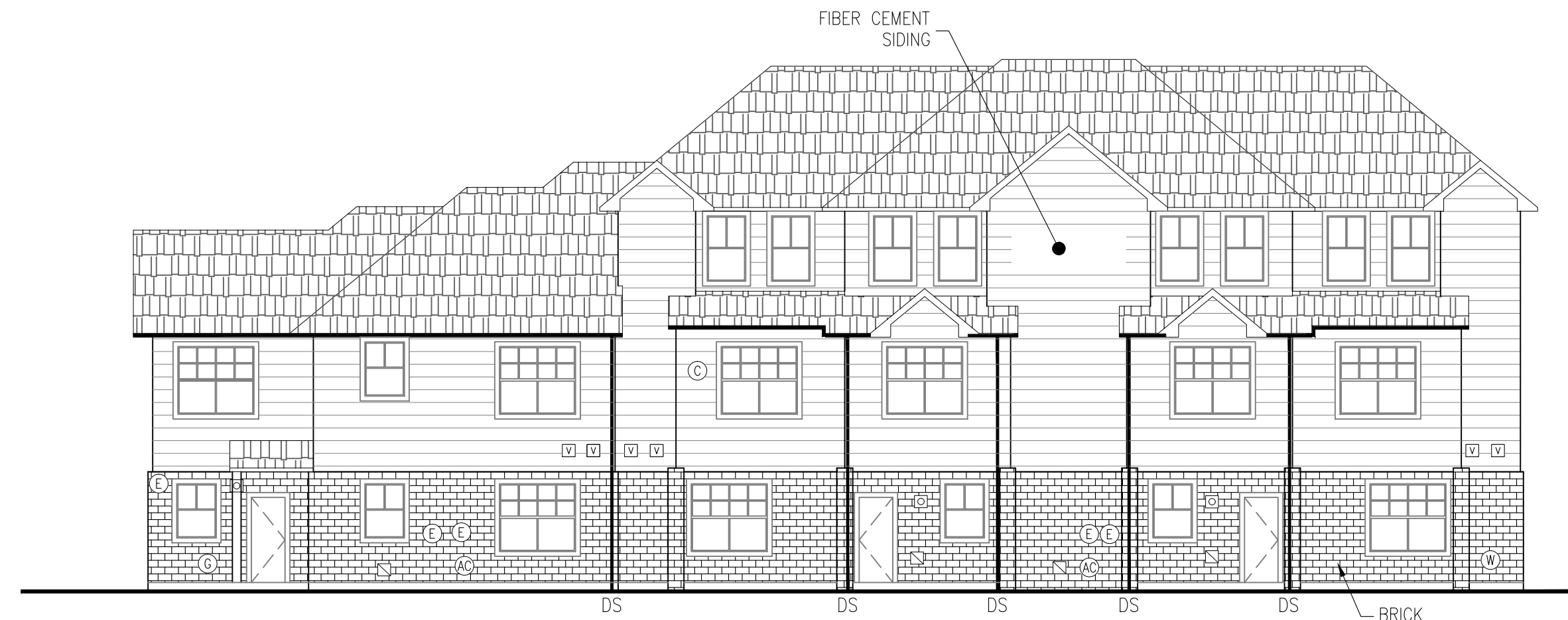
② BUILDING 18 REAR ELEVATION R3.15 NTS
