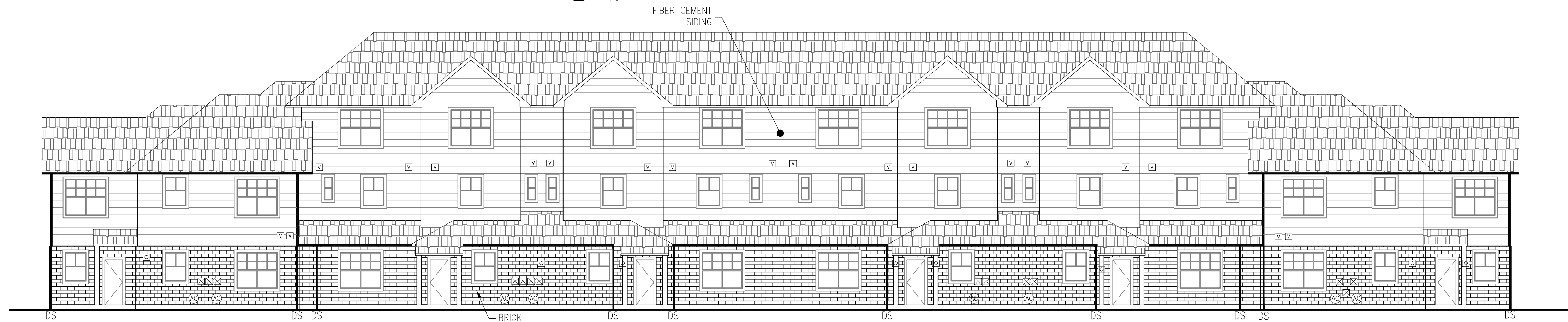
② BUILDING 6 REAR ELEVATION R3.03 NTS
