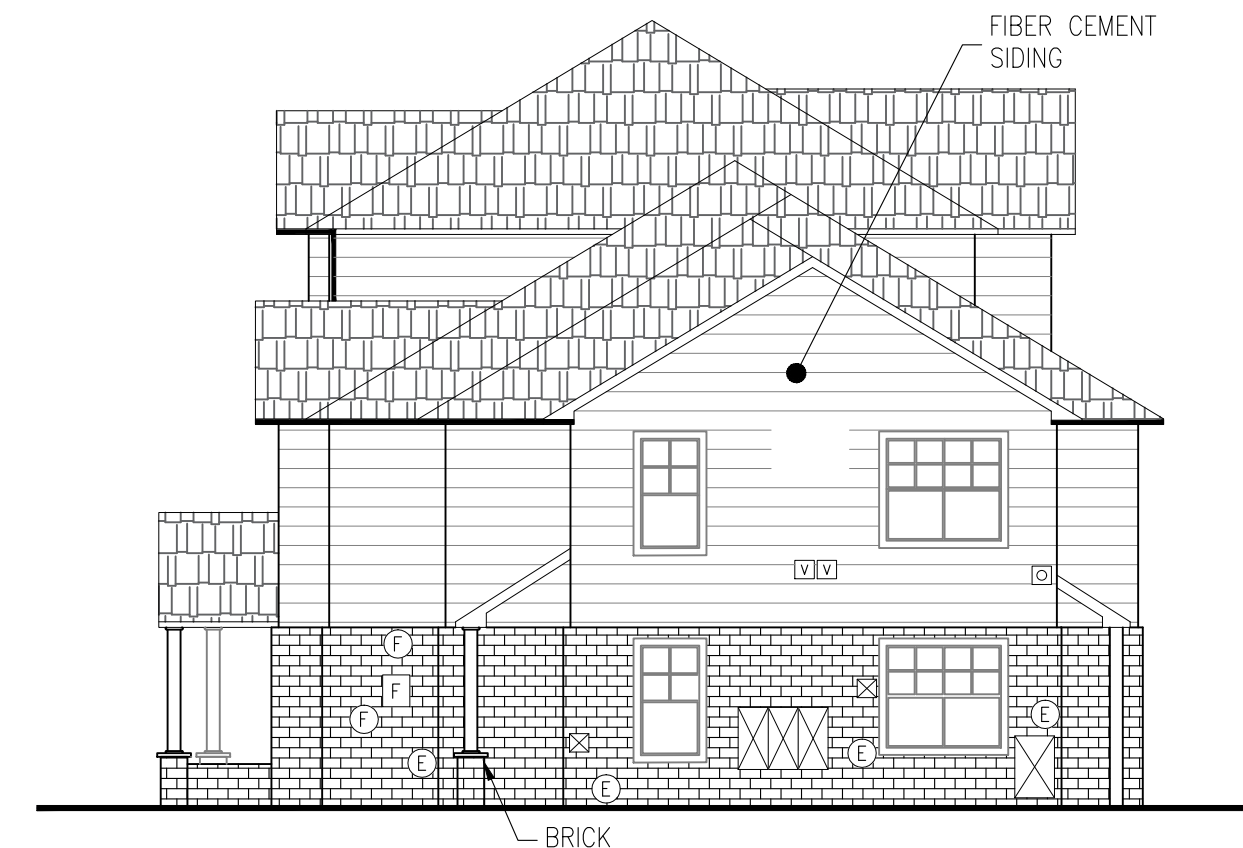
④ BUILDING 14 SIDE ELEVATION
