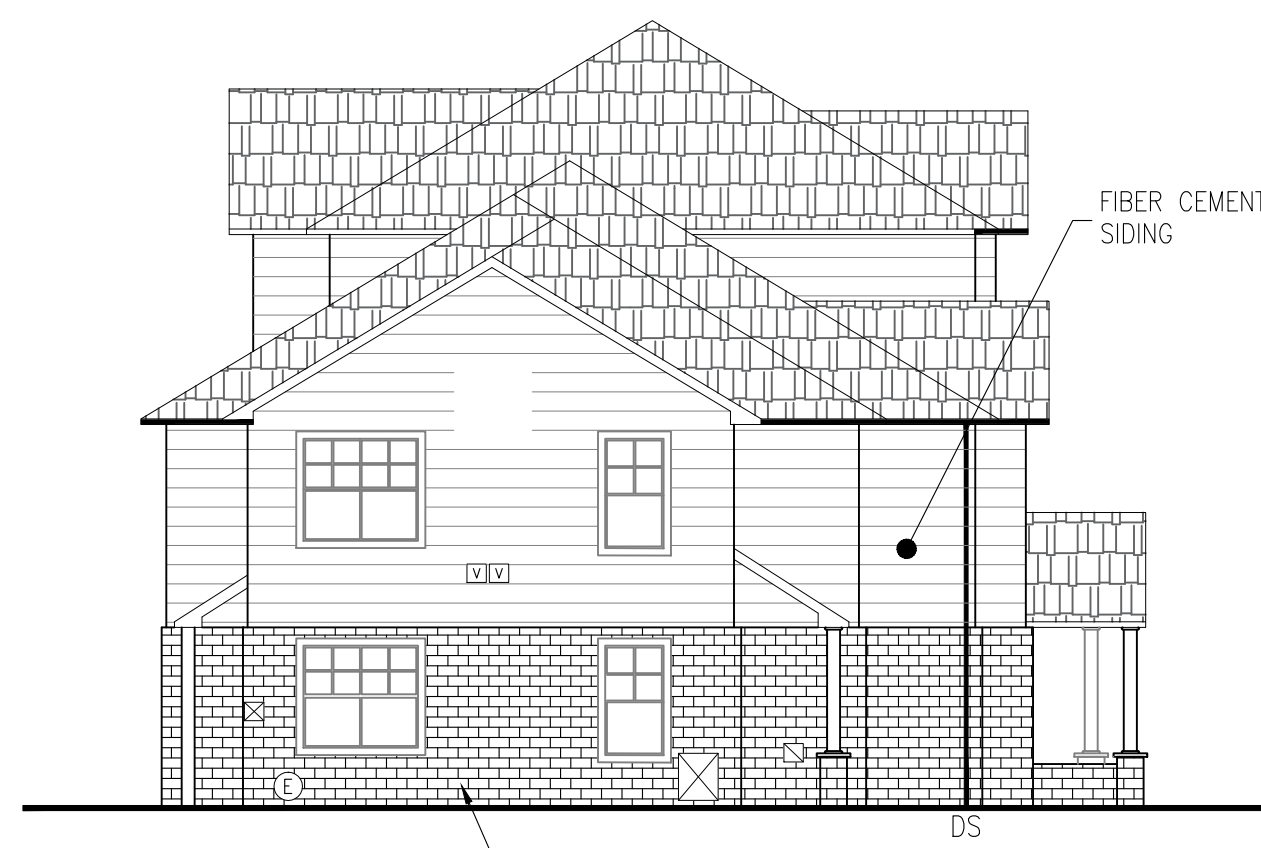
③ BUILDING 14 SIDE ELEVATION
